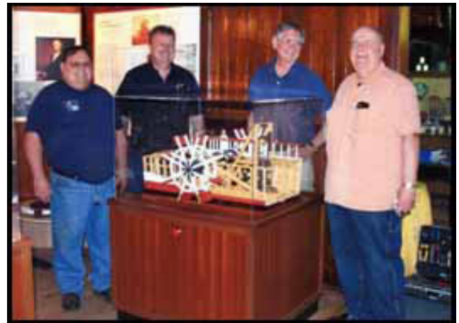
Animated 1/12th scale model of Robert Fulton's Clermont Running gear. It demonstrates how the steam Engine turns the paddle wheels
